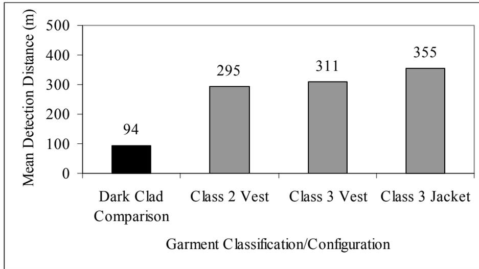
Figure 4. The main effect of garment classification/configuration on conspicuity.
