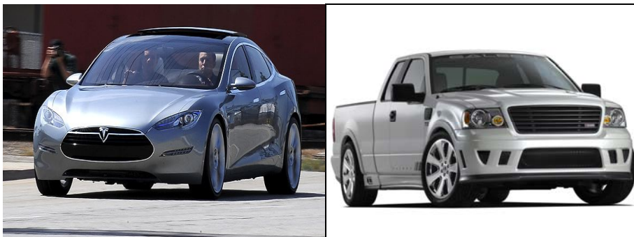
Figure A-2 – Group/Level 1 Vehicles, Car and Truck with Eye to Headlamp Distance about 0.5m
