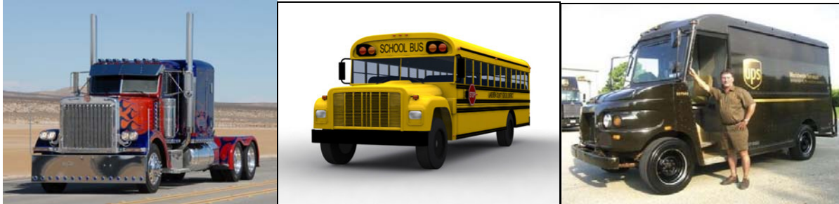
Figure A-3 – Group/Level 2 Vehicles, Truck and Bus with Eye to Head Lamp Distance about 1.2m
