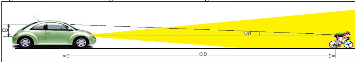
The distance from driver’s eye to vehicle’s head lamp, ED, varies. For most passenger cars, the average ED is 0.5 meter, as shown in two vehicles in Figure 2.
